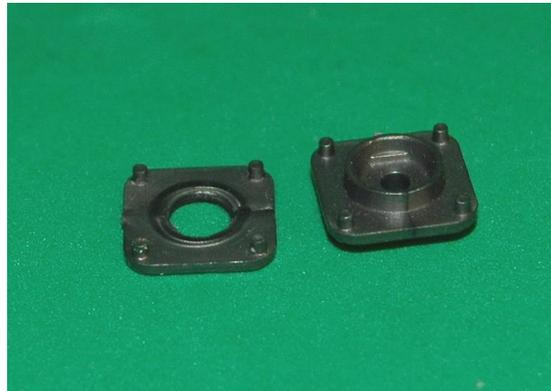
Then take part # "B52" and remove the "Boss" on the outer face and drill out the hole in the center with a 4mm diameter drill. That will remove the "Boss" on the backside at the same time.
